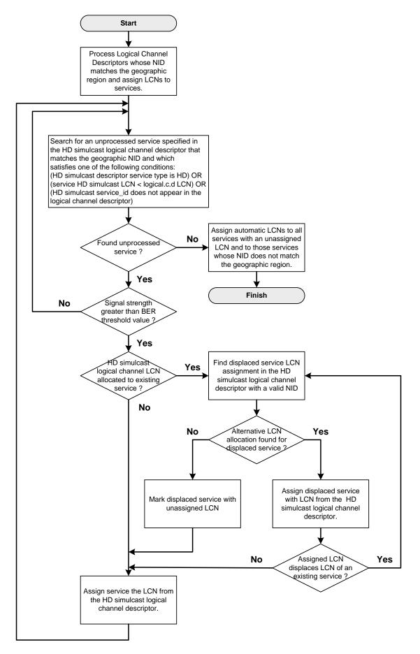
Figure 6: HD\_simulcast\_LCN operation
