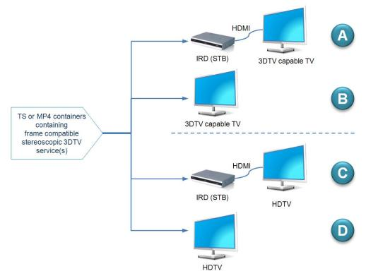
Figure 13: Frame compatible plano-stereoscopic 3DTV IRD use cases
