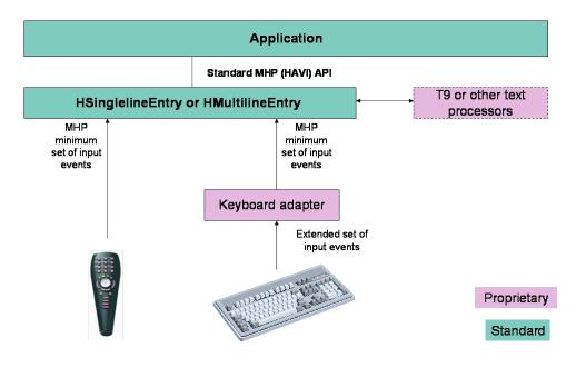
Figure 5: Text Entry Layering Schematic
